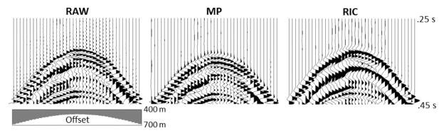
Figure 3 First arrivals at early times showing ringyness in the RAW and MP data sets. The RIC dataset has only slight ringyness.
