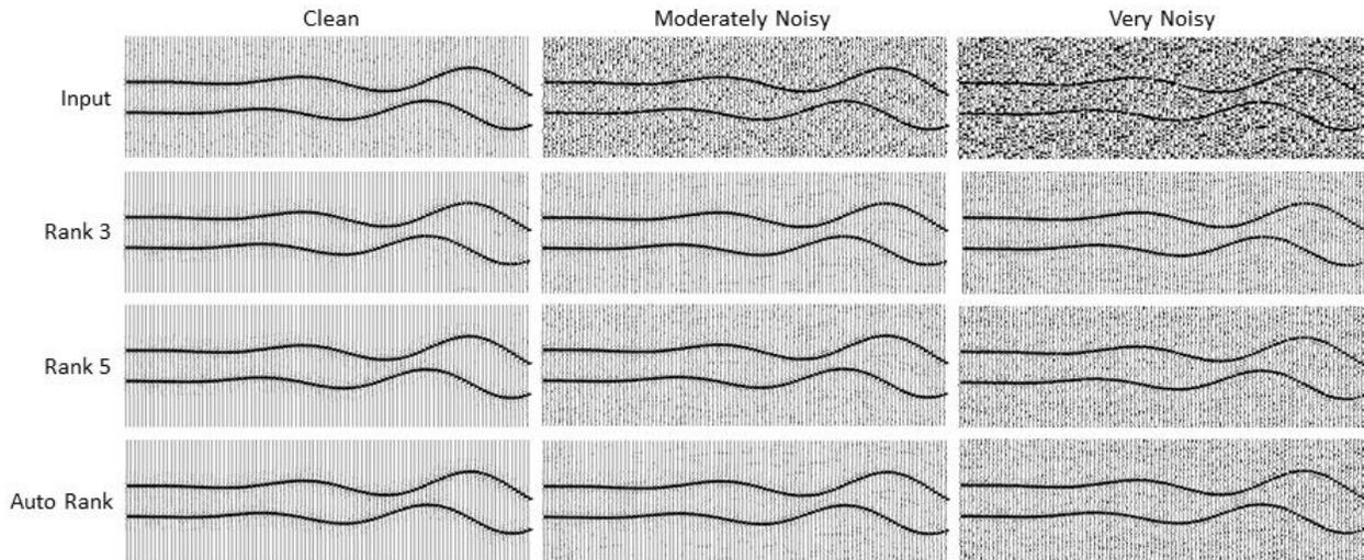
Figure 3: Synthetic tests 400 ms in the time direction. The three raw horizontal slices are shown along the top. Below these are f-xy Cadzow filtered versions with rank 3, rank 5, and automatic rank determination with threshold capping.
