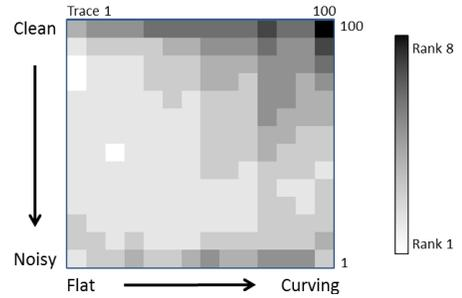
Figure 2: Automatically determined rank averaged over 15 to 70 Hz. The rank increases as the section gets cleaner and more structured. The effects of threshold capping are seen at the bottom.
