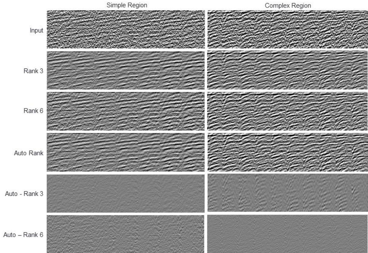
Figure 5: Two different regions of NMO-corrected cross-spread gathers from a real 3D data set. In the simpler region on the left, f-xy Cadzow with automatic rank determination behaves like a rank-3 filter, giving more aggressive noise suppression than rank 6. In the more complex region on the right, automatic rank determination behaves like a rank-6 filter, preserving coherency better than rank 3.
