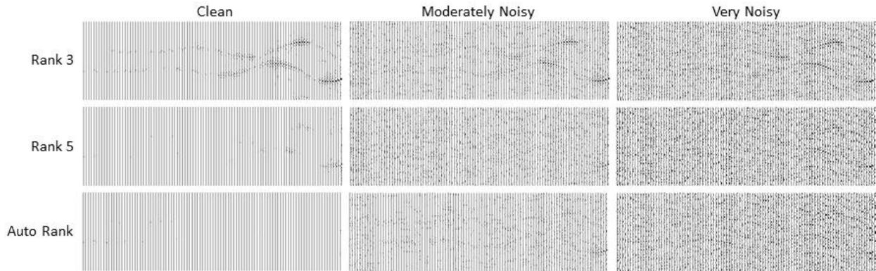
Figure 4: The difference between the noiseless signal and the various filtered versions of the noisy data from the previous figure. Automatic rank determination has removed the least amount of signal while suppressing more noise than the rank-5 filter in the flatter regions.
