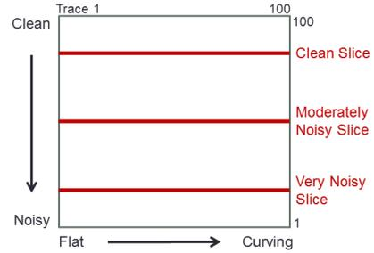
Figure 1: 100 x 100 synthetic trace grid. Event curvature increases from left to right, and noise amplitude increases from top to bottom. Three horizontal trace slices (shown in red) are analyzed.
